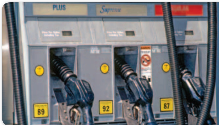
■ Figure 21.8 Octane ratings are used to give the antiknock rating of fuel. Mid-grade gasoline for cars has an octane rating of about 89. Aviation fuel has an octane rating of about 100. Racing fuel has an octane rating of about 110.
